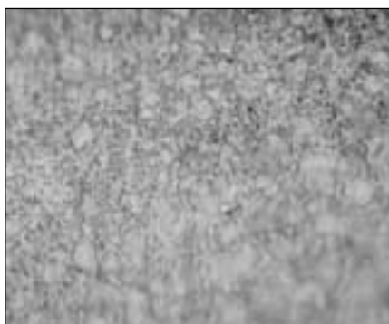
Fig. 4 - Formulation 1, 24-hour water-exposed surface; 40 F (4 C) cure; 850X, brightfield
