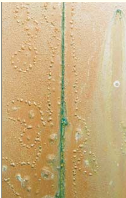
Fig. 1 - Electroendosmotic blistering around a cut scribe and discrete corroding points.
