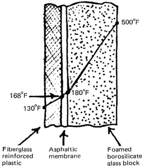
**Figure 17-2:** Foamed borosilicate glass block and urethane asphalt adhesive/membrane over fiberglass reinforced plastic.
