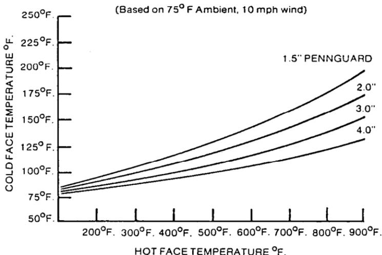
**Figure 17-1:** Temperature gradient for various thicknesses of foamed borosilicate glass block.
