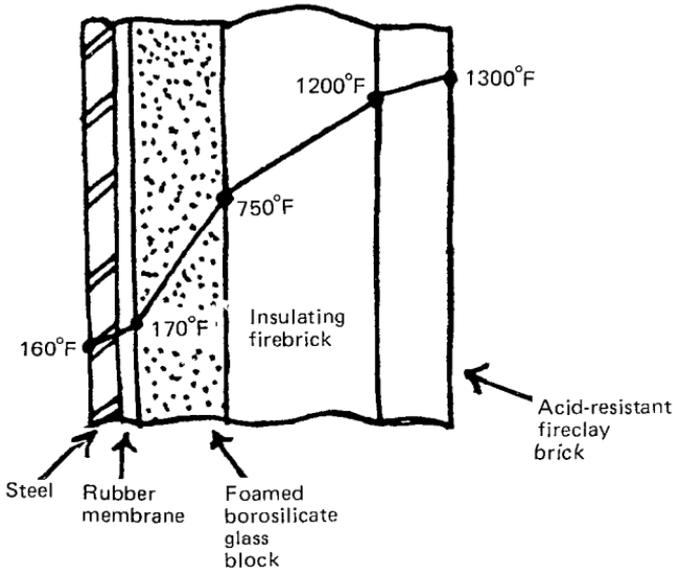
**Figure 17-3:** Combination lining incorporating foamed borosilicate glass block reduces courses of brick required to lower temperature to acceptable level at the membrane.
