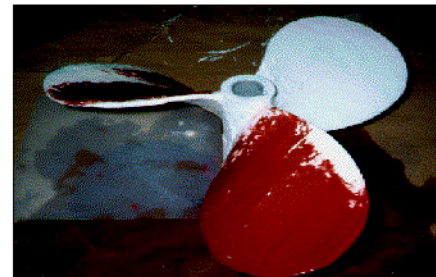
Application of TS-RB rebuilding compound
