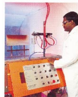
Figure 10. Comparative chip resistance test (ASTM D-3170-87) of an epoxy amine coating with KEVLAR® and with fumed silica.
