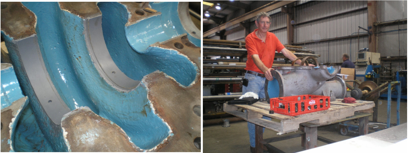
A New Valve and Impellor are blasted and coated with ARCOR EE-11 Prime and ARCOR S-20.
