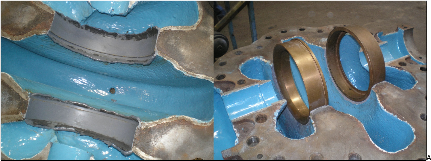
A New Agitator is blasted and coated with ARCOR EE-11 Prime. ARCOR EE-92 was added to increase wear resistance/life. The ARCOR EE-11 Prime is then hand rubbed to 'slick out' the EE-92 prior to final coating with ARCOR S-20.
