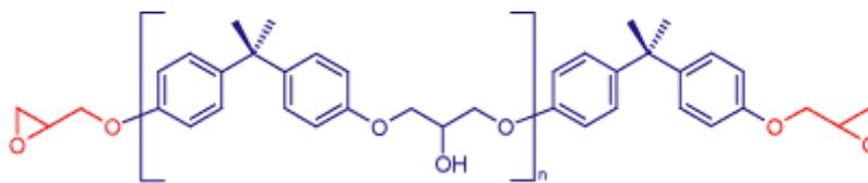
**Figure 1:** Structure of DGEBA resin
