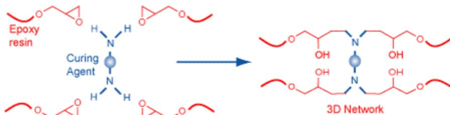
**Figure 2:** Curing mechanism of Epoxy resins
