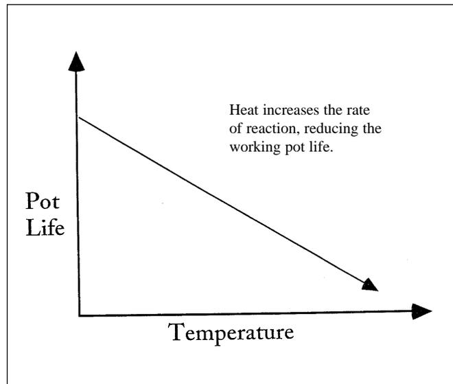
Fig. 5: Applying heat to a plural component coating often shortens pot life or speeds curing.
