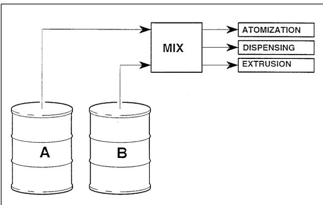
Fig. 1: The basic sequence in the use of plural component coatings
