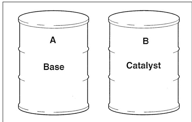
Fig. 2: The base and catalyst of a plural component coating are commonly referred to as Component A and Component B.
