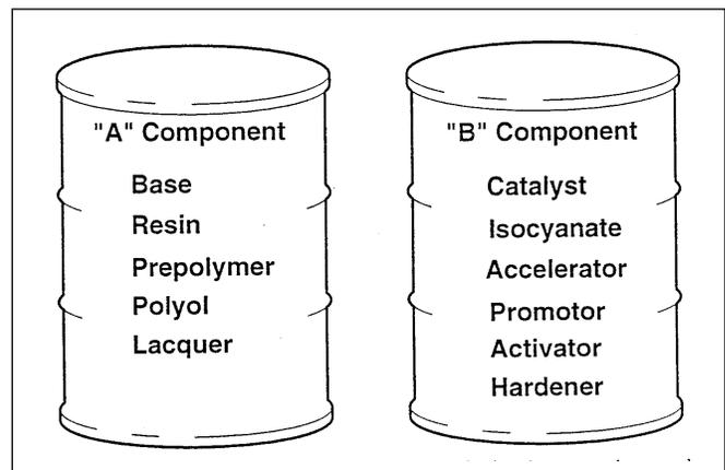
Fig. 3: Other terms used to describe Component A and Component B
