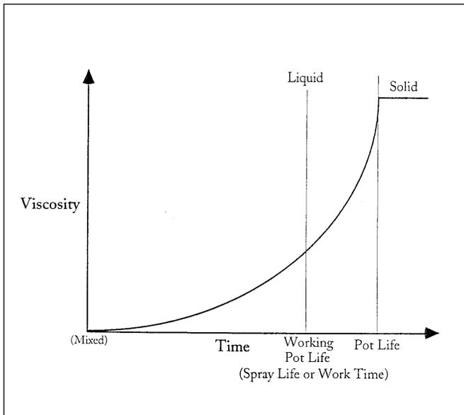
Fig. 4: As time passes, the pot life of a plural-component coating decreases.
