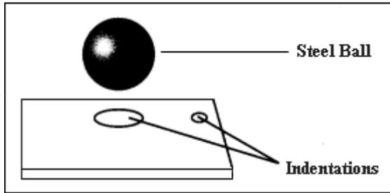
The results obtained from this test are useful measures of relative resistance to indentation of various grades of plastics. However, the Rockwell hardness test does not serve well as a predictor of other properties such as strength or resistance to scratches, abrasion, or wear, and should not be used alone for product design specifications.
