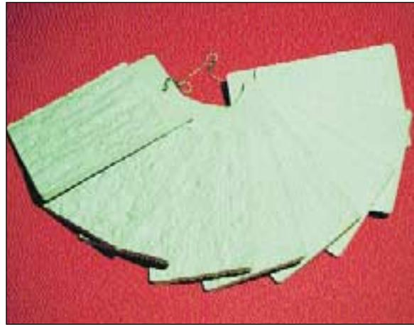
**Figure 2 — Replicas of different surface profiles for concrete substrates**
